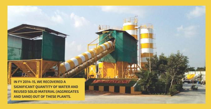
At present, UltraTech has 62 concrete recycling plants across India. In FY 2014-15, we recovered a significant quantity of water and reused solid material (aggregates and sand) out of these plants. The water removed out of it was put to use in concrete production and some internal consumption after the sedimentation process.
