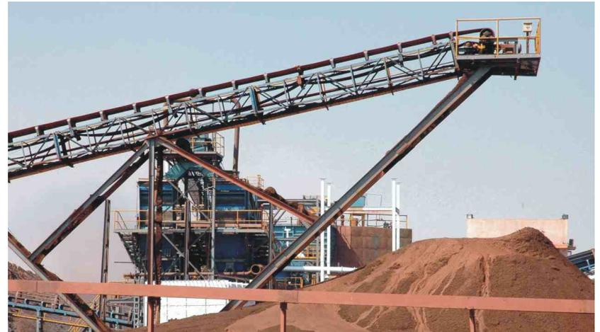
We have mechanised our mine and have adopted state-of-the-art technology which reduces manual intervention during mining activities. The down hill conveyor system has reduced the need for ore transportation from the mine area to the loading station through road, thus reducing air pollution as well as diesel usage in trucks. Moreover our dependence on road transportation has further been reduced by switching over to the rail mode.
