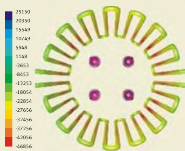
CFD results depicting contour of heat flux (W/m 2 ) along tube wall
